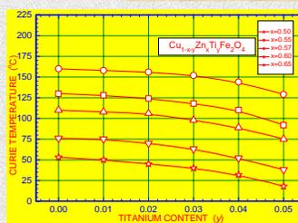
Fig. 4. Effect of composition on  $T_c$  of some CuZnTi ferrites
