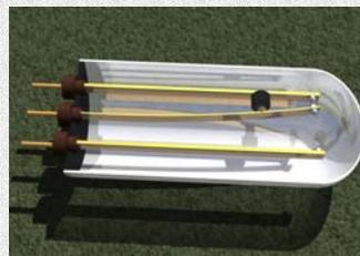
Fig. 9a. Cross section in the thermomagnetic relay
