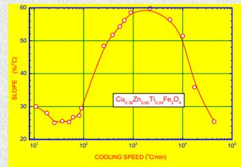
Fig. 6. The dependence of the slope of  $\mu(T)$  curves on the cooling speed for one composition of CuZnTi ferrite
