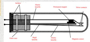
Fig. 9b The main elements of the thermomagnetic relay
