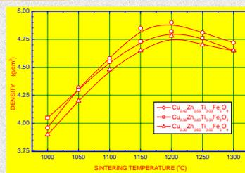
Fig. 3. The density behavior with sintering temperature for three compositions of CuZnTi ferrite
