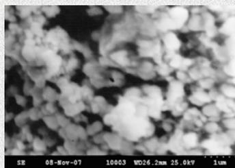
Fig. 2. SEM image of the morphostructure of the milled powder of the CuZnTi ferrite
