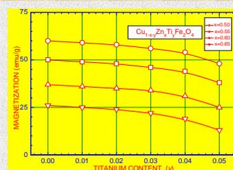
Fig. 5. Effect of composition on magnetization of some CuZnTi ferrites
