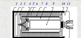
Fig. 7a: 1- outer metallic case; 2- electronics; 3- protective disc; 4- coil; 5- magnetothermal sensor; 6- thermal isolating blanket; 7- heating resistance; 8- hollow thermostat body; 9- thermostat chamber; 10- protective disc; 11- external connector.
