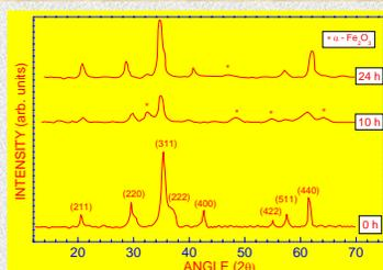
Fig. 1. X-ray diffraction patterns of CuZnTi ferrite
