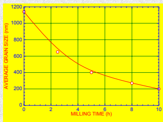
Fig. 2. Average grain size of iron doped \text{TiO}_2 as a function of the milling time.
